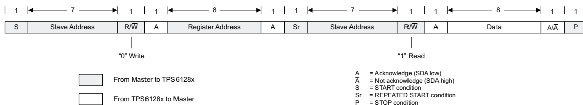
Figure 50. “Read” Data Transfer Format in Standard-, Fast, Fast-Plus Modes
